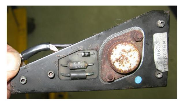
Here the diode has been replaced (almost any diode will do, in this case we use a 1N4001). Note that the cathode band is towards the pointed end of the controller.
