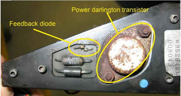
Note feedback diode is broken. This is very common and is due to water ingress. Also common is for one of its leads to corrode-Though. Occasionally the power darlington transistor can fail. Use MJ11016 as replacement.
